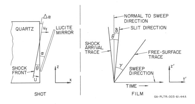
Fig. 2.5.--Definition of Parameters Used in Adjusting Streak Camera Data.
